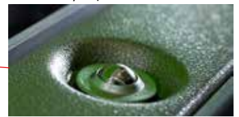
Ball transfers in back gauge table (nylon balls as option)
