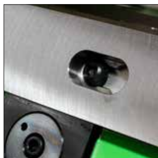
Quick change tooling (bayonet style) and adjustable crowning.
