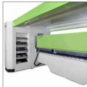
Folding beam in upper position before clamping.
